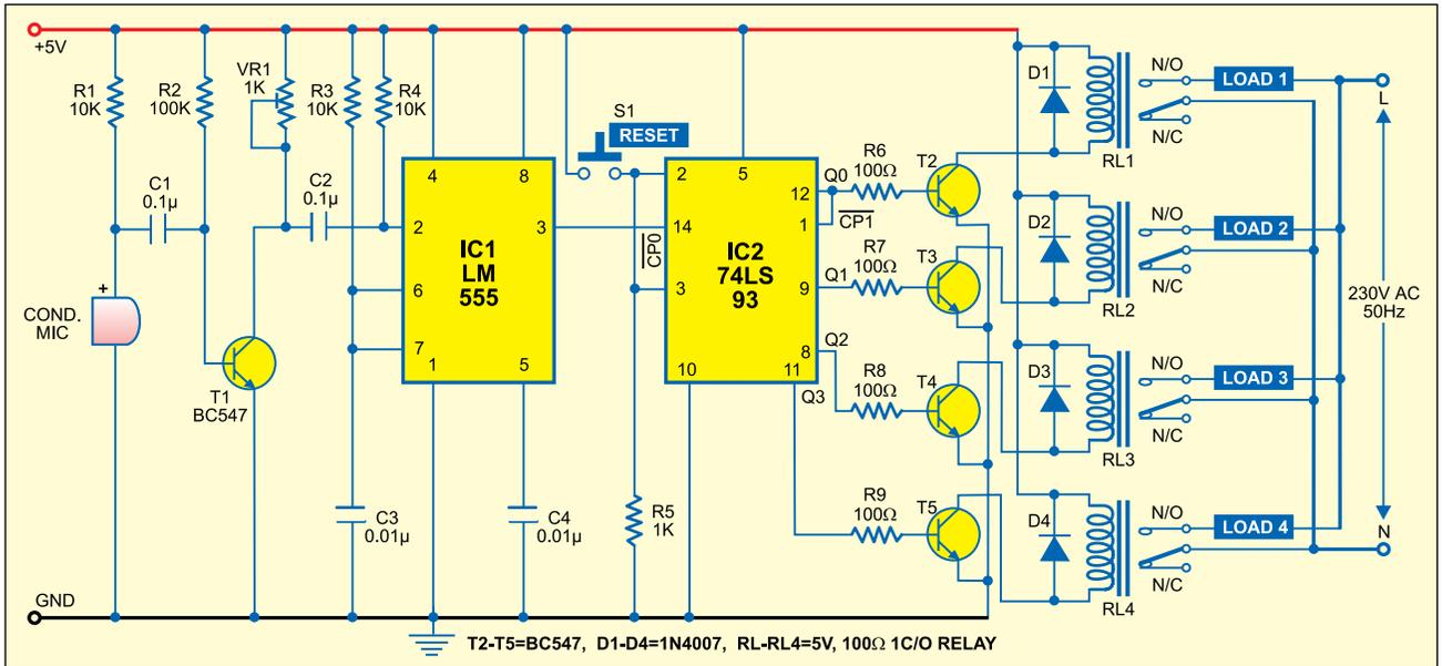
used in this circuit, which you can keep by the bedside. You can switch on/off up to four different electrical equipment (TV, fan, light, etc) in 16 different ways.
